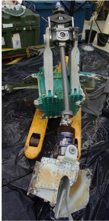
Figure 61: Trimmable horizontal stabiliser screwjack after being raised on board
