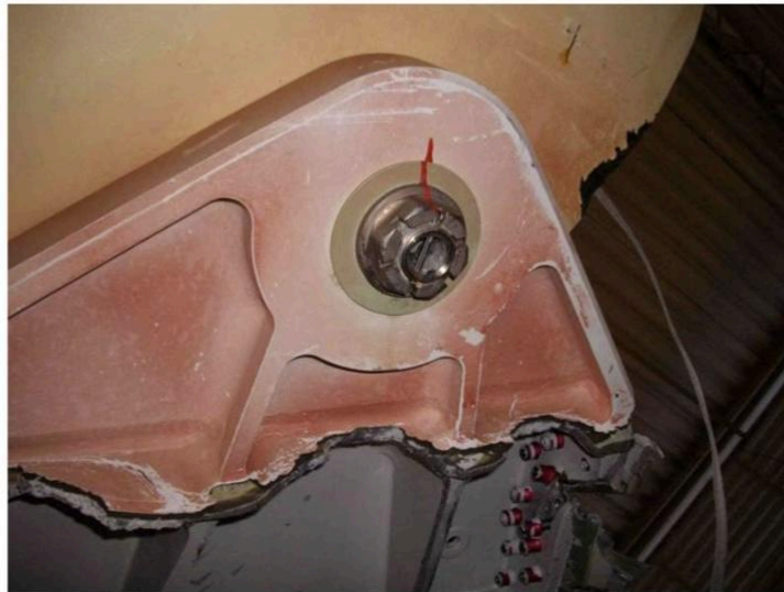
Figure 49: Right-hand aft lug: shearing of the fuselage along main frames 86-87
