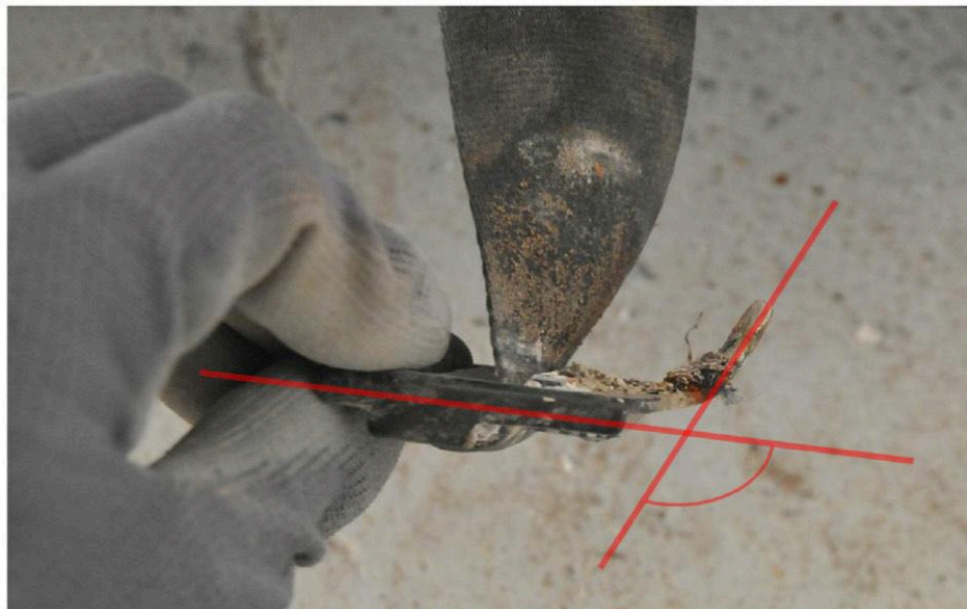
Figure 84: Malformation of the crotch belt fastening
