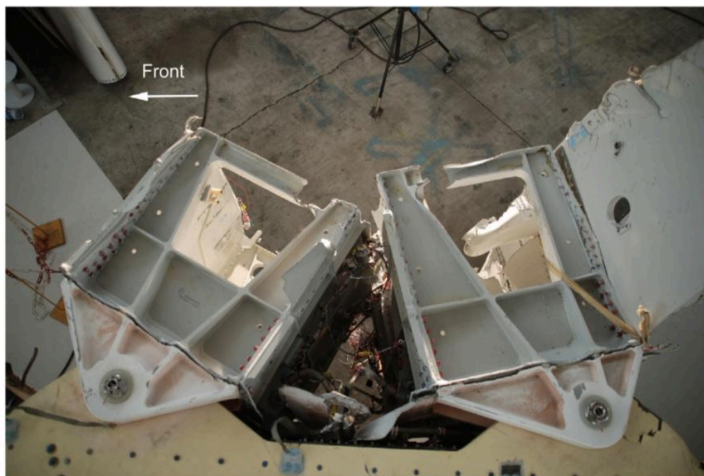
Figure 51: Fin centre and aft attachments
