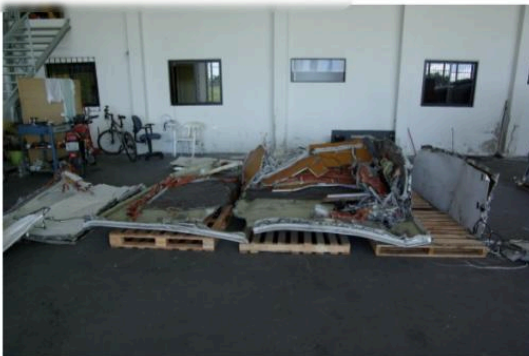
Figure 38: Floor of the LDMCR: with bottom-upwards deformation
