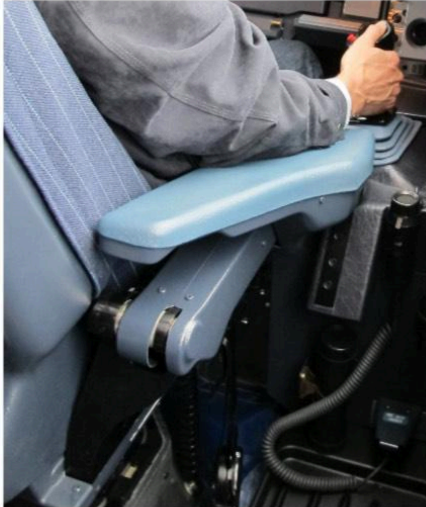
Figure 79: Right seat armrest on the side-stick side
