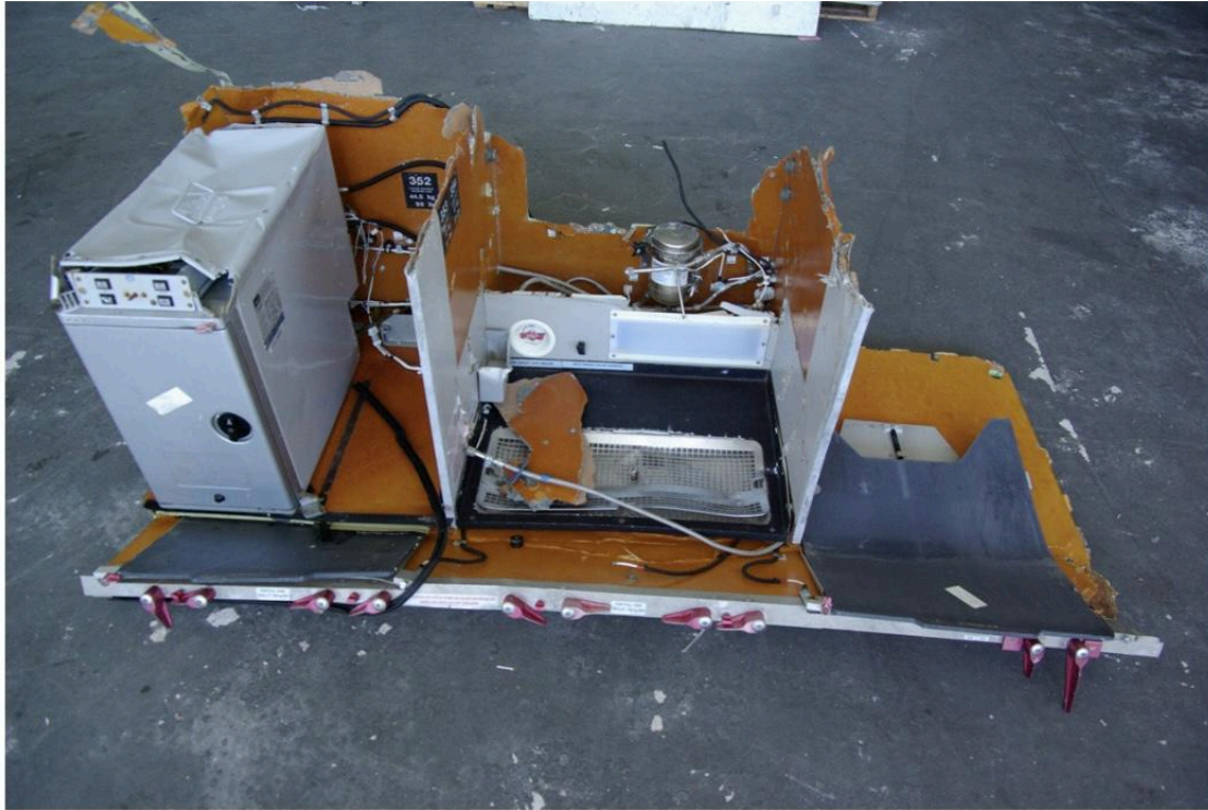
Figure 35: Part of Galley G3: downwards deformation at the level of the galley's heavy parts
