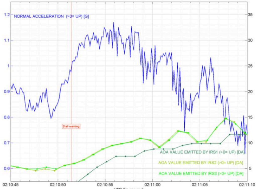
Figure 66: Evolution of normal acceleration recorded at the time of activation of the stall warning
