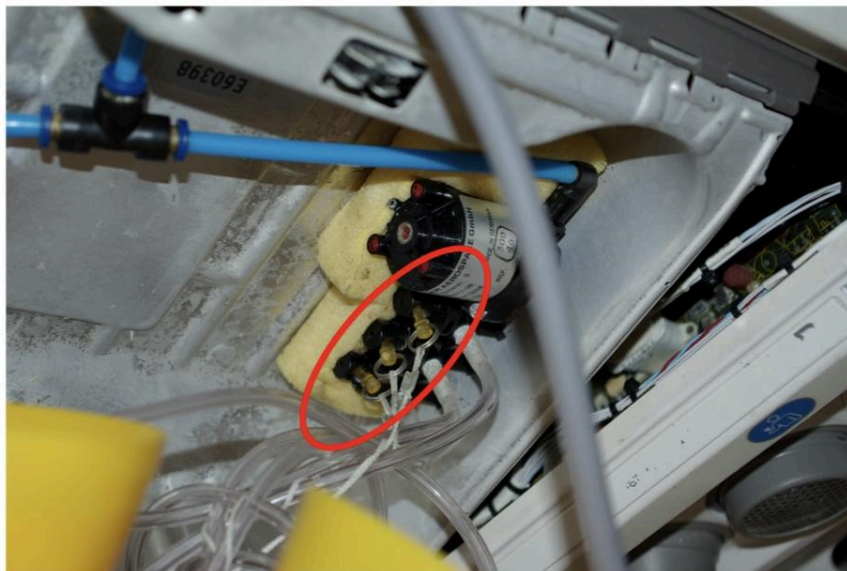
Figure 41: Passenger oxygen container recovered open: the three pins are in place
