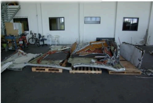
Figure 38: Floor of the LDMCR: with bottom-upwards deformation
